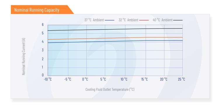
The level of performance provided by each machine depends on the conditions at which it is operating. The two factors determining performance are ambient air temperature and the required cooling fluid outlet temperature. The above graphs illustrate the cooling capacity and nominal running current – at three different operating ambient temperatures – based on differing cooling fluid outlet temperatures.
