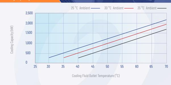
The level of performance provided by each machine depends on the conditions at which it is operating. The two factors determining performance are ambient air temperature and the required cooling fluid outlet temperature. The above graph illustrates the cooling capacity achieved at three different operating ambient temperatures – based on differing cooling fluid outlet temperatures.
