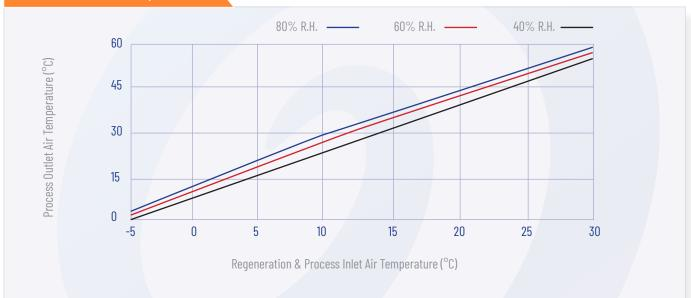
The level of performance provided by each machine depends on the conditions at which it is operating. The factors determining performance are the temperature & relative humidity (R.H.) of the inlet air. The above graph illustrates the dehumidifying capacity – at three different R.H. levels – based on differing inlet air temperatures.
