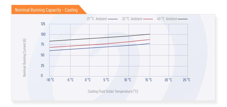
The level of performance provided by each machine depends on the conditions at which it is operating. The two factors determining performance are ambient air temperature and the required heating / cooling fluid outlet temperature. The above graphs illustrate the heating / cooling capacities and nominal running current – at three different operating ambient temperatures – based on differing fluid outlet temperatures.
