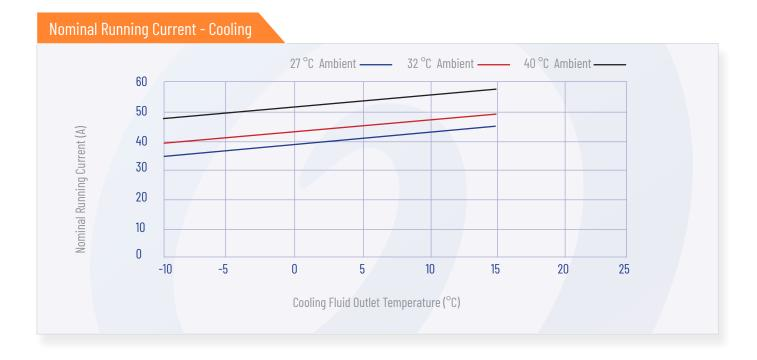
The level of performance provided by each machine depends on the conditions at which it is operating. The two factors determining performance are ambient air temperature and the required heating / cooling fluid outlet temperature. The above graphs illustrate the heating / cooling capacities and nominal running current – at three different operating
