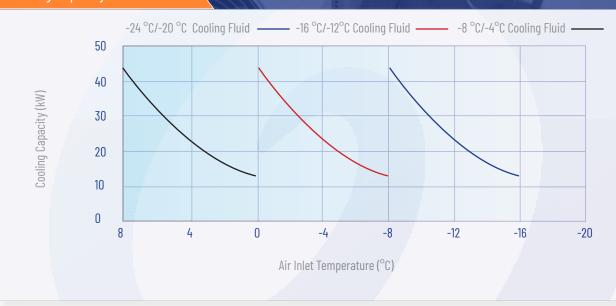
The level of performance provided by each machine depends on the conditions at which it is operating. The two factors determining performance are ambient air temperature and the required cooling fluid outlet temperature. The above graph illustrates the cooling capacity achieved at three different sets of cooling fluid temperatures – based on differing ambient temperatures.
